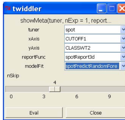
Figure 4: The user interface in tdmPlotResMeta . The user may select the tuner, the design variables to show on x- and y-axis, the display function ( spotReport3d or spotReportContour ) and the metamodel function ( modelFit ). Two optional sliders are nExper and nSkip (see text).
