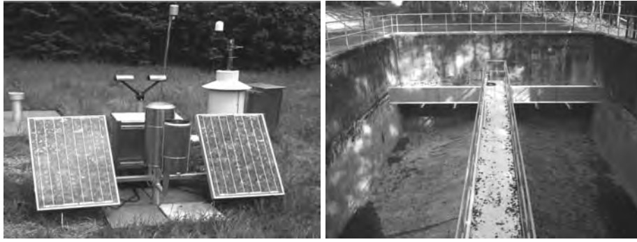
Figure 1: Left: rain gauge (pluviometer). Right: stormwater tank.
