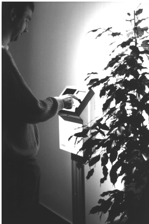
Fig. 2. The access control system ZN-Face in a prototype realization, consisting of camera (behind semi-permeable mirror), LC-display and card reader.
