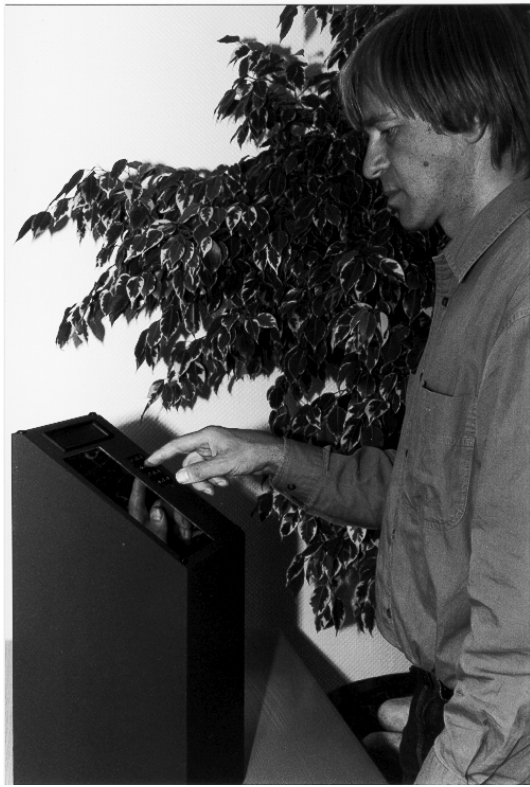
Figure 2: The access control system ZN-Face in a prototype realization, consisting of camera (behind semi-permeable mirror), LC-display and PIN pad.
