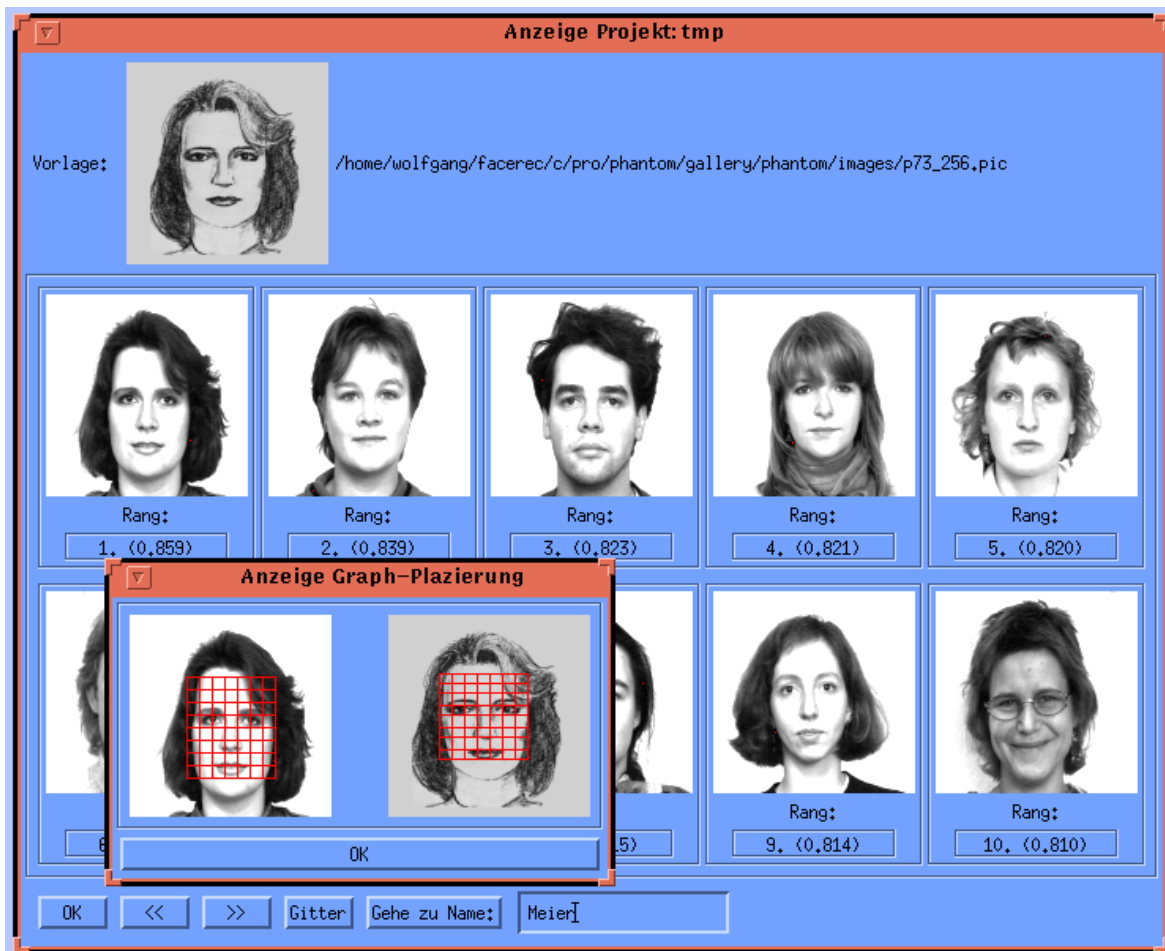
Fig. 2. The result of a PHANTOMAS search on a line drawing (upper left) where the true match is found at place 1 of the ranking list. The small inset shows how the graphs are positioned on the faces in order to account for the different size and aspect ratio.
