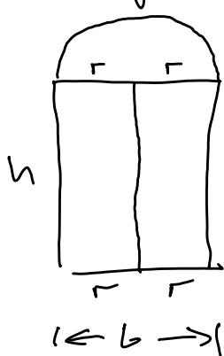
$$(*) \text{ Umfang } U = \underbrace{2r}_{\text{unten}} + \underbrace{2h}_{l/r} + \underbrace{\frac{2\pi r}{2}}_{\text{Bogen}} = 20$$
