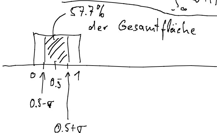
$$\begin{aligned} \text{Normalverteilung } w(f) &= \frac{1}{\sigma\sqrt{2\pi}} \exp\left(-\frac{(f-\mu)^2}{2\sigma^2}\right) \\ &= \frac{1}{\sigma\sqrt{2\pi}} e^{-\frac{(f-\mu)^2}{2\sigma^2}} \end{aligned}$$
